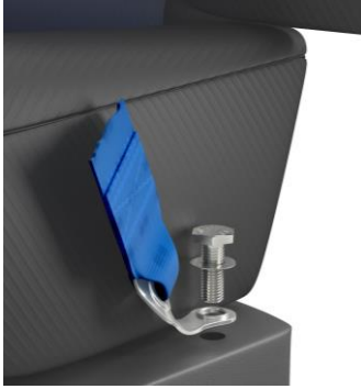
Installation without stock belts for rear seats.
