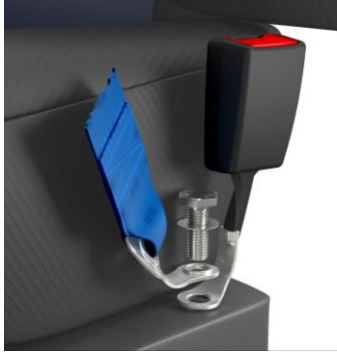
Installation with stock belts for rear seats.
