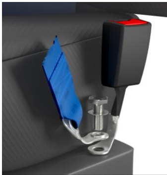
Installation with stock belts for rear seats.
