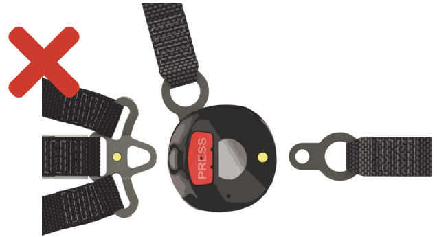
this figure shows the wrong installation of the right 5 Point Net Buckle System 09577
