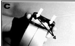
Figure C: Keep the metal retainer positioned between your thumb and forefinger. Slide the plastic cover backwards onto the metal frame as indicated until both ratchets [4] locks with a distinct clicking sound into the deepenings at the metal frame.
