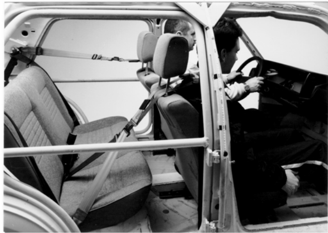
Only the passenger seat is equipped with a SCHROTH Rallye 4 harnessbelt system!
