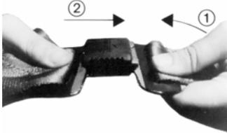
To open: Slide the plastic cover in the direction of the arrow to the stop (1). Tilt the latch downwards and remove it from the buckle (2).
